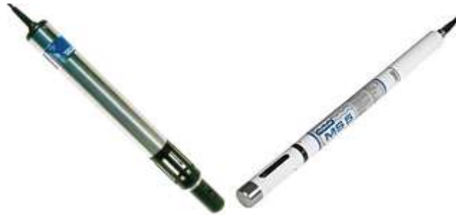
Figure 10. Pictures of the water quality probes used in this study, with the Greenspan CS304 (left) and the Hydrolab MS5 (right).
